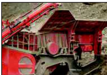
Hopper and Feeder
