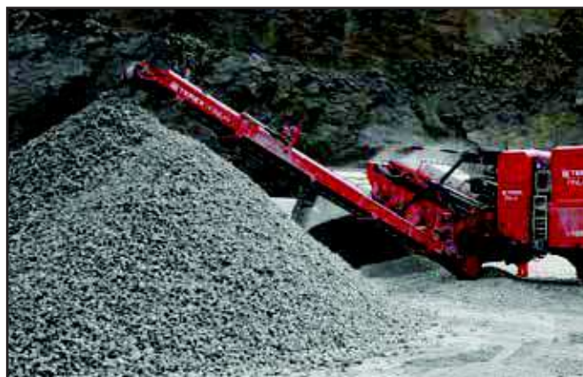
Re-circulating conveyor (stockpiling mode)
