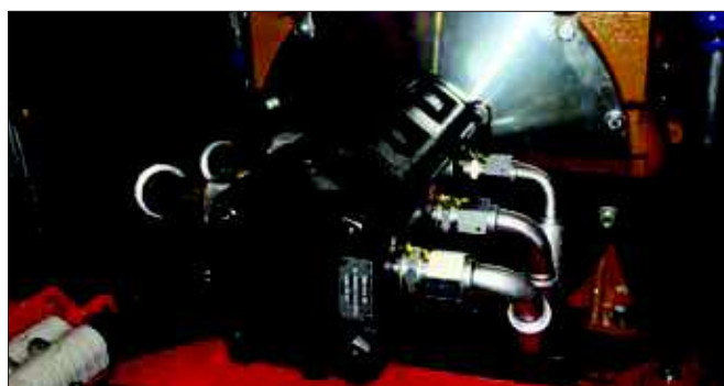
Pump 1: Triple 33cc/rev, 33cc/rev, 26cc/rev
