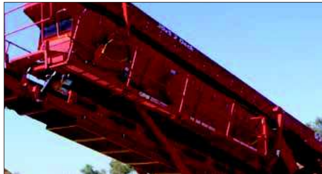
Screenbox with all round catwalk access
